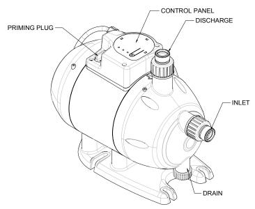
The Mach 5 is a compact and powerful water pressure system comprised of a water-cooled motor, integrated flow and pressure control, and a quiet multi-stage self-priming pump. An inlet check valve is incorporated into the suction port. A control panel at the top of the pump provides status information, dry tank protection, and reset capability.
